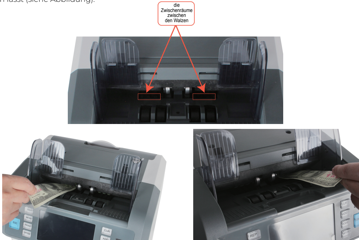
One banknote to check the gap between the rollers.
